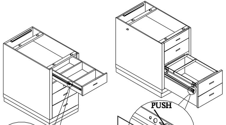
Press the left side plastic up, and press the right side plastic down, then pull out the drawer.
