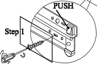
Remove the screw on the bottom slide away push the plastic inside then pull the drawer out.
