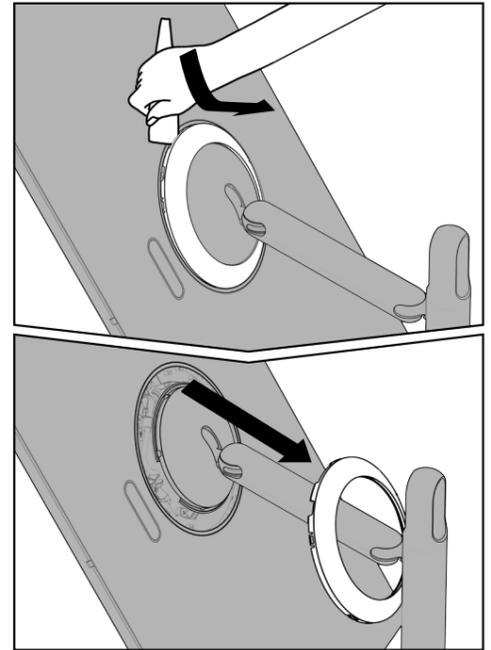
**4** Position the screen horizontally and disassemble the cable holder screw.
