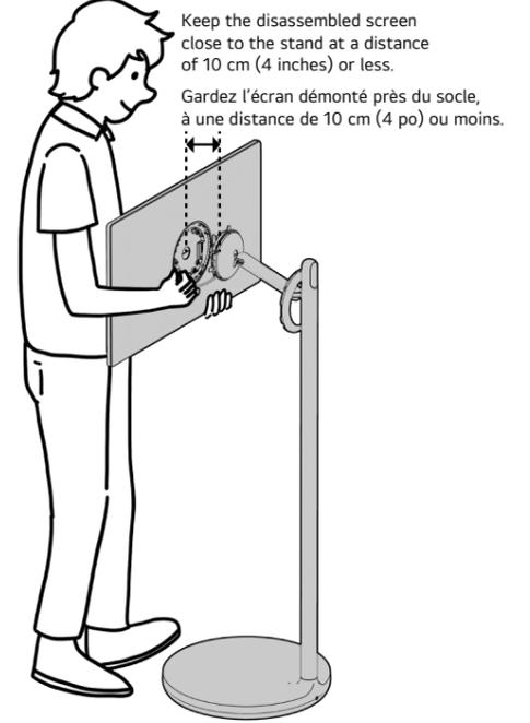
Keep the disassembled screen close to the stand at a distance of 10 cm (4 inches) or less.
