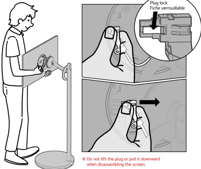
※ Do not lift the plug or pull it downward when disassembling the screen.
