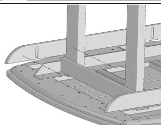
Align Long Aprons with Aluminum Support Brace. Ensure that pockets in Long Apron are aligned with Screws used to attach Short Aprons. Secure using (12) 3/4" Pan Head Screws thru Aluminum Support Brace.
