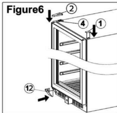
**6.** Replace the upper hinge (4) with the screws (3a). Insert the locking cap (6), screws (7) and (8) and attach the hinge cap (2). Replace the hinge cover (1) and the lower hinge cover (12).
