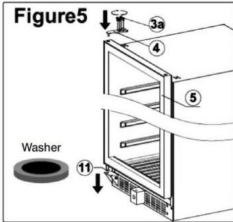
**5.** Place the washer (11) on the metal hinge pin (9) and replace the door on the bottom hinge by aligning the metal hinge pin (9) with the outer hinge hole on the bottom hinge (10).
