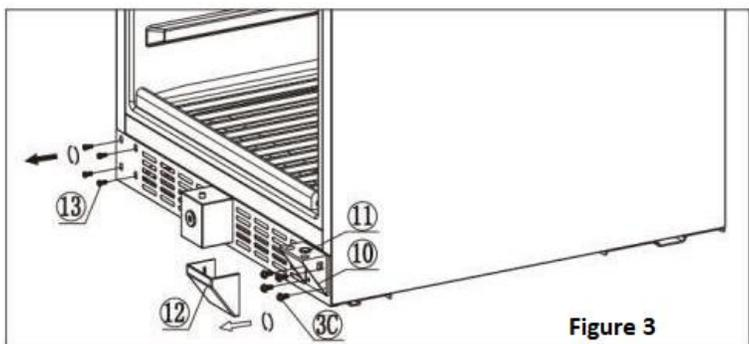
**3.** Using a flat-head screwdriver, lift off the lower hinge cover (12). Using a Phillips head screwdriver, loosen and remove screws (3c) and (13) and lower hinge (10)
