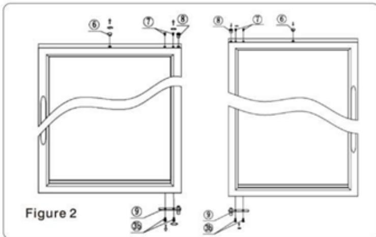
**2.** Using a Phillips head screwdriver, loosen the screws (3b) to remove the metal rod from the hinge (9) at the bottom of the door. Turn the door 180° (clockwise) so that the top is now the bottom and vice versa. Attach the metal rod of the bottom hinge (9) to the bottom corner of the door and secure it with the screws (3b).
