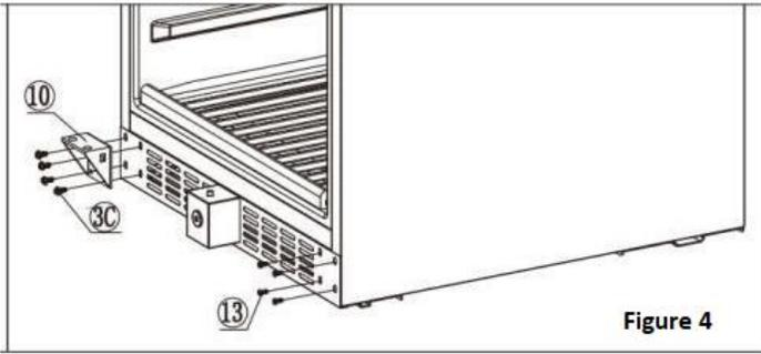
**4.** Move the lower hinge (10) to the opposite side and re-insert all screws (3c) and (8). The lower hinge cover (12) must fold over the lower hinge (10).
