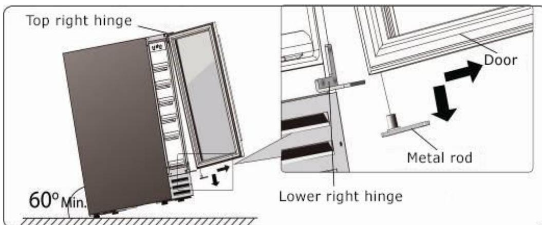
**3.** Use a small flat head screwdriver to lift and remove the plastic cap on the upper center (locking hole) of the door and insert it into the lower center hole, rotate the door 180 degrees (counterclockwise) so that the top becomes the bottom.
