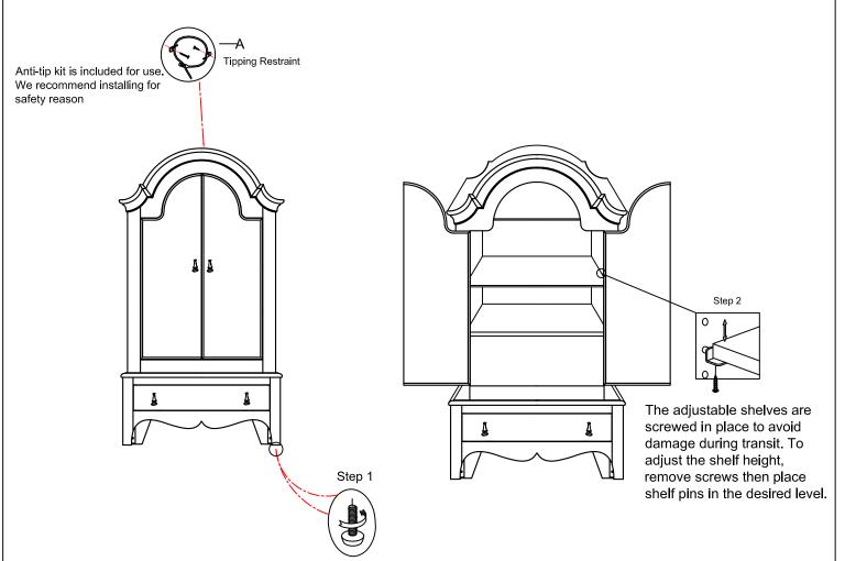
Adjust Leveler if needed to level case on uneven floor.
