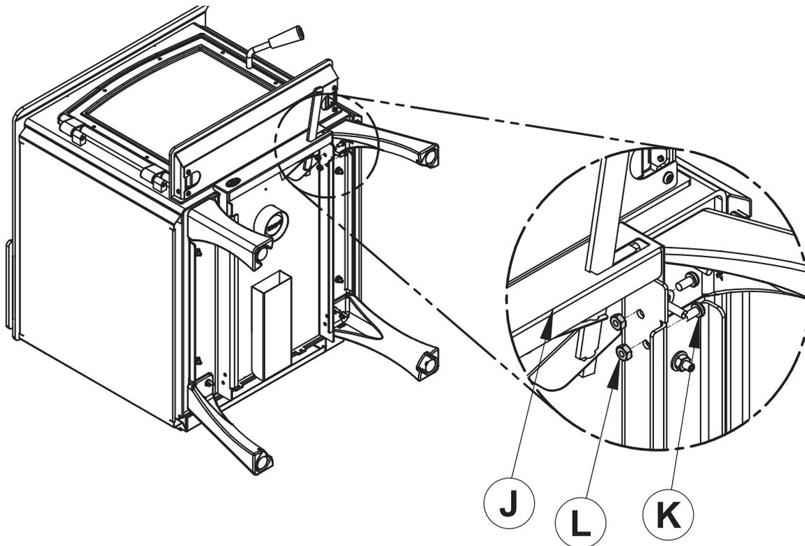
6. Put the stove on its legs, install the ash drawer included with the kit. Put back the firebricks, the ash plug and the door on the stove (See step 1).
