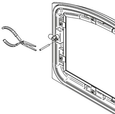
Figure 26: Removing the split pin
