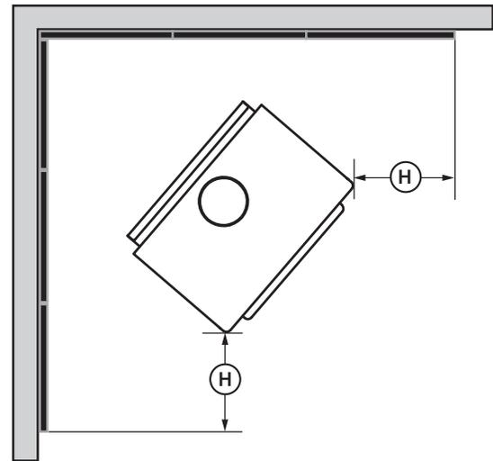
Figure 25: Heat shield clearances
