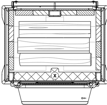
Figure 12: Position of the bottom pieces (High burn)
