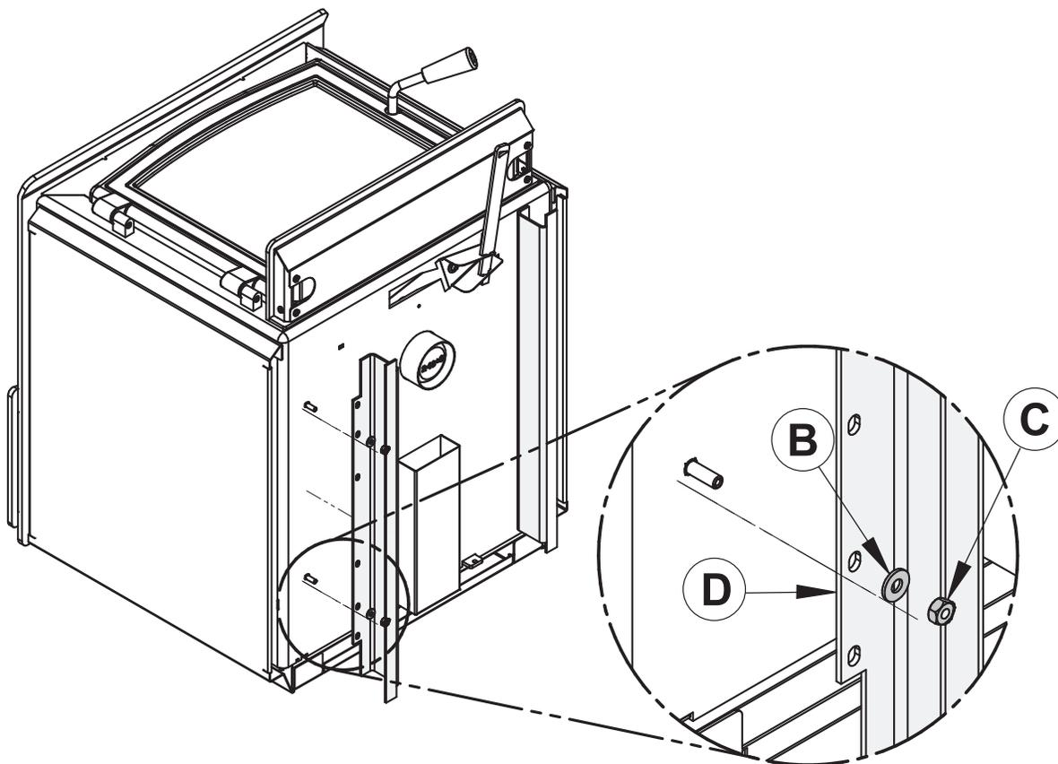
3. Install the pedestal (**E**) on the stove and screw it in place using washers (**B**) and nuts (**C**).
