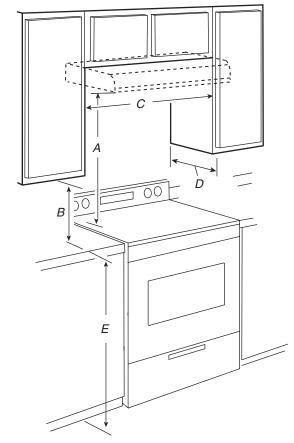
A. 18" (45.7 cm) minimum distance from electric cooking surface. 24" (61.0 cm) minimum distance from gas cooking surface. 30" (76.2 cm) suggested maximum above the cooking surface.
