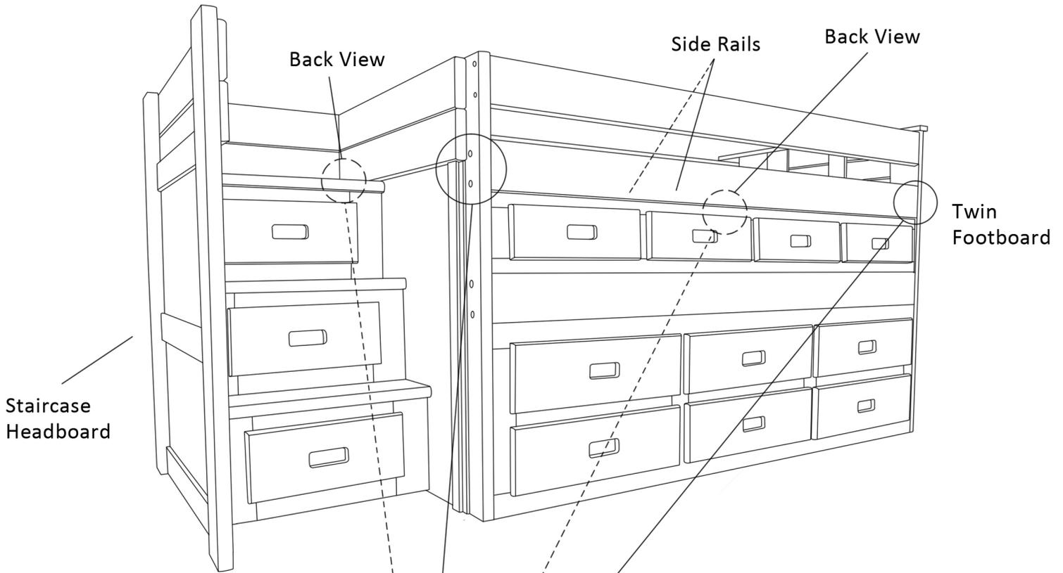
1) Align two side rails to the holes of the Twin Footboard and Staircase Headboard as indicated in the diagram. Insert bolts (#B) to the holes of the side rails connecting to the Twin Footboard and Staircase Headboard from the inside view.
