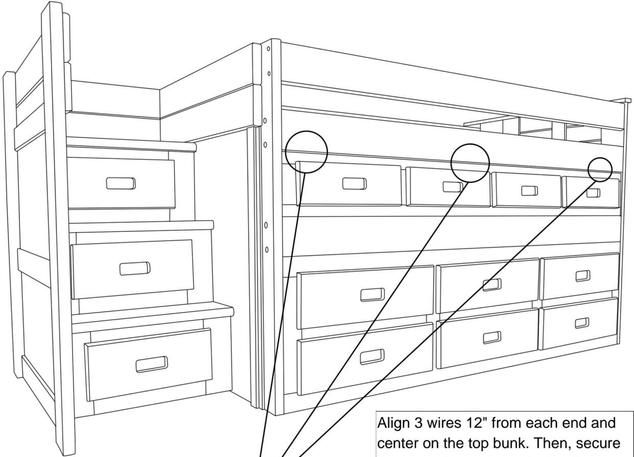
Align 3 wires 12" from each end and center on the top bunk. Then, secure screws (#A) as shown in the diagram.
