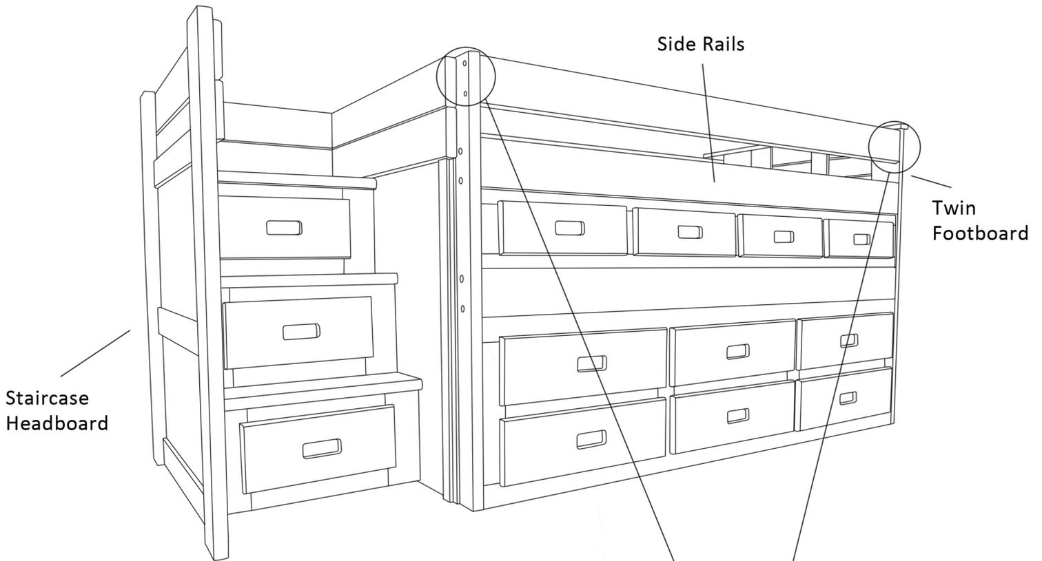
Align two guardrails to the holes of Staircase Headboard and Twin Footboard, then secure by using screws (#D).
