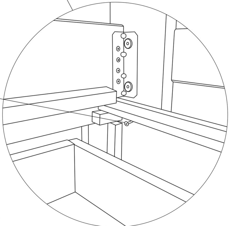
Have another person screw screws (#F) from the inside view of the four drawer unit, to the HB/FB and staircase. Each upper four corners from the inside view of the four drawer unit to HB/FB and staircase should be secured with a screw
