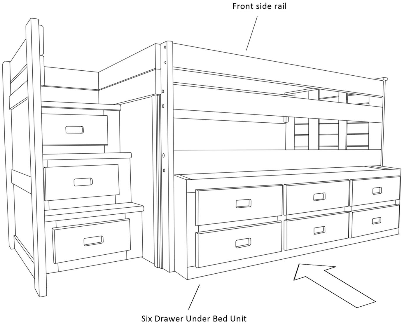
Carefully slide Six Drawer Under Bed Unit to the inside bottom of the day bed frame. Make sure the six drawer unit is aligned with the front side rail.
