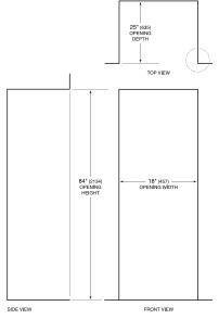
NOTE: 31/2\* (89) finished returns will be visible and should be finished to match cabinetr
