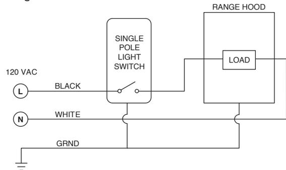
4. Mount single pole toggle light switch in switch box.
