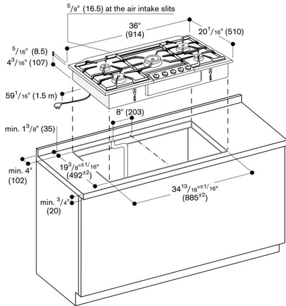
Minimum distance from the appliance cut-out to the side wall 11 3/16" (300 mm).
