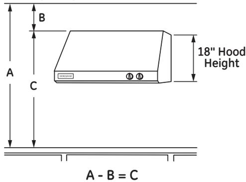
We recommend that the vent hood and decorative duct cover (if used) be on site before final framing and wall finishing. This will help to accurately locate studs, ductwork and electrical service.
