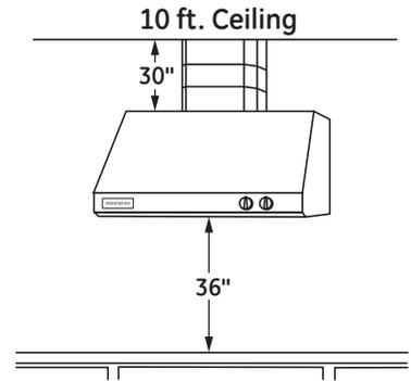
**10 ft. ceilings:** When the hood is installed 36" above the cooking surface, order three 12" and one 6" duct cover accessories.
