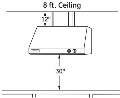
**8 ft. ceilings:** When the hood is installed 30" above the cooking surface and there is no soffit or upper cabinetry, order one 12" duct cover accessory.
