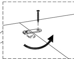
**STEP 1:** Take off one screw from each mounting plate and swing it to the proper location on the other bookcase before re-securing it with the screw.
