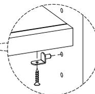
If you prefer to adjust the shelf location, remove the screws and move shelf brackets to the desired location. Then secure the brackets to shelf with screws.
