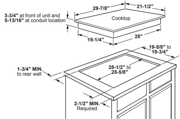
To insure accuracy, it is best to make a template when cutting the opening in the counter
