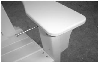
Arms should be installed with curve side on the inside of the chair. (Left Picture). Place Arm on top of Front Leg. Align pre-drilled hole in arm with the pre-drilled hole located at the top of the Front Leg. Install a 3-1/2" connector bolt through pre-drilled hole in the Front Leg, then through pre-drilled hole under arm. Install flat washer, lock washer and nuts. Do not tighten at this time. Repeat process on other side.
