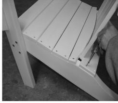
Place Back Assembly on top of mounting surface of Rear Legs, (Left Picture). Push Back Assembly forward until it's aligned with Seat Assembly. Hold Back Assembly in place and install (4) 1-3/4" Phillip's Head Screws into pre-drilled holes on each side.
