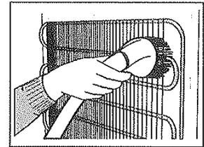
**CAUTION:** Failure to unplug the unit could result in electrical shock or personal injury.
