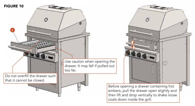
Use caution when opening the Hybrid Fire Grilling Drawer. It is possible to pull it all the way out of the grill, and there is no stop mechanism to prevent it from coming all the way out.
