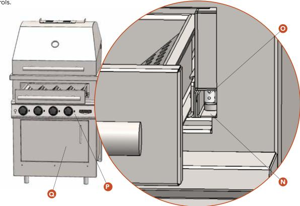
**Q.** Access Doors: The cabinet below the grill is not for storage. This space contains the cleanout pan and the electrical system for the grill. Never store combustible materials inside this cabinet or any items that may be damaged by heat. The rotisserie spit and forks may be stored inside the cabinet. Never attempt to store a LP cylinder underneath the grill.
