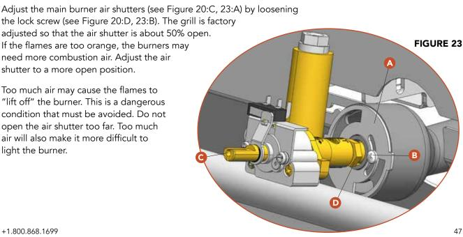
Reinstall the burner into the grill, being careful to ensure the burner is seated properly over the orifice (Figures 20:E and 23:D) and the locating posts (Figure 20:F) are seated into the burner support brackets. Test the burner on HIGH for proper flame characteristics before reinstalling the burner guard.
