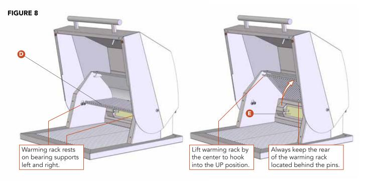
**E.** Rotisserie Burner(s): Infrared burners for optional use with rotisserie spit system. Rotisserie cooking can be done using heat from the rotisserie burner(s) OR heat from below. *NEVER operate rotisserie burner(s) at the same time as the main burners or other heat source below.*
