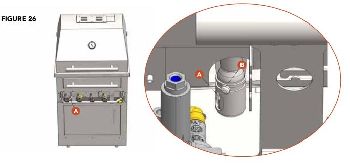
Loosen the screw that secured the air shutter (see Figure 26:B). Use care not to remove the screw by loosening too far. Adjust the air shutter until the flames burn blue, are stable, and do not lift off the burner. Secure the air shutter in position by re-tightening the screw.
