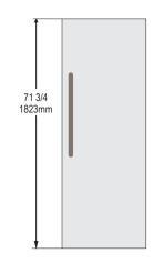
Custom panels should be at least 5/8"(16mm) and a maximum of 3/4"(19mm) thick and they should cover the front of the dedicated cabinet box.
