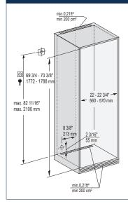
This is a fully integrated refrigerator appliance designed to be completely enclosed in a dedicated kitchen cabinet. This dedicated cabinet box must be constructed in accordance with the specified dimensions and must allow for sufficient air circulation to ensure proper operation. For more details about ventilation requirements, please refer to Design Guide.
