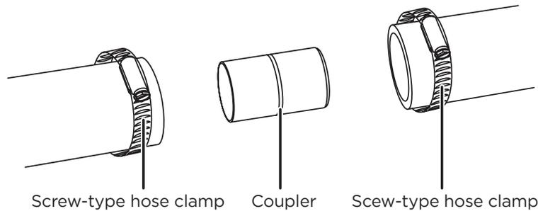
**3** Secure the drain hose to the air gap, waste tee, or garbage disposal with a screw-type clamp, using the appropriate method below. **See "Drain preparation" on page 6**, if you do not know which method to use.
