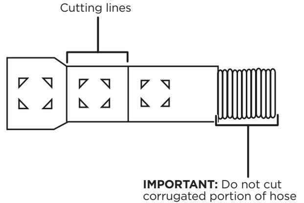
**IMPORTANT:** For proper drain operation, the total drain hose length must not exceed 10 ft. (3.01 m).
