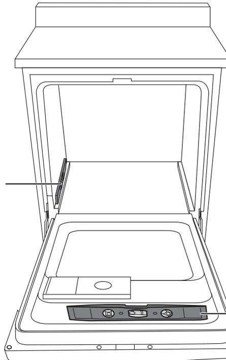
**2** Level the dishwasher by adjusting the four leveling legs individually.
