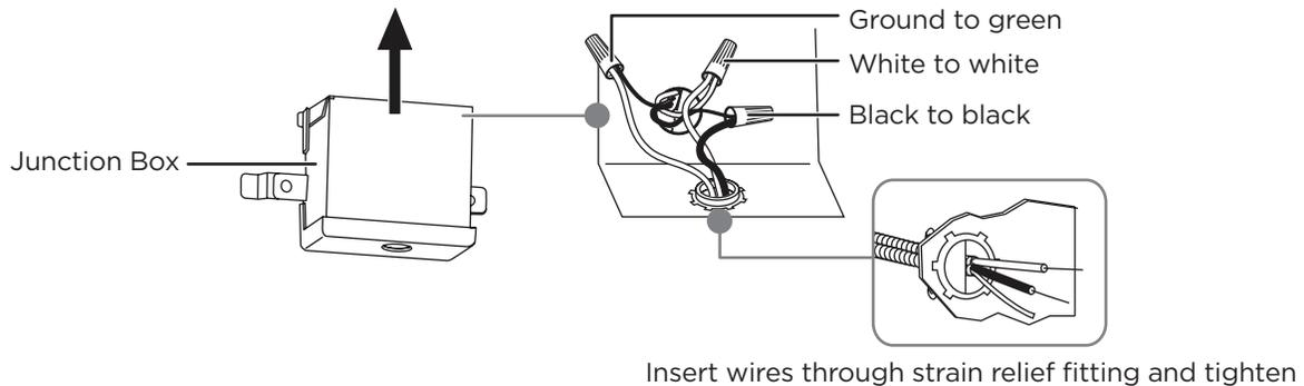
2 Locate the three dishwasher wires, (white, black, and green) with stripped ends, then insert the dishwasher wires through the small hole in the junction box.
