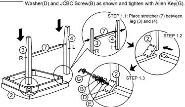
STEP 1: Assemble each leg (3) and (4) to seat (2) with Flat Washer(E), Spring
