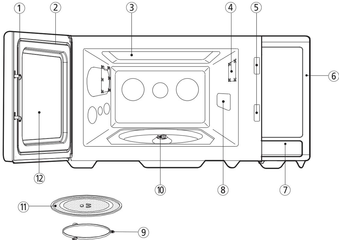
① **Door latch** - When the door is closed, it will automatically shut off. If the door is opened while the oven is operating, the magnetron will automatically shut off.
