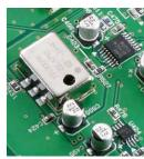
audio playback. The cornerstone of quality sound, its large crystal element realizes both excellent center accuracy (±0.5ppm, as shipped from the factory) and extremely low levels of phase noise to ensure exceptional sound playback quality.
