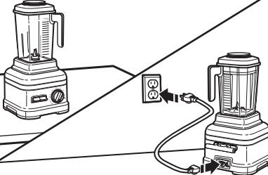
Before using the Blender, be sure the countertop beneath the Blender and surrounding areas are dry and clean. Be sure the power switch on the back of the blender base is in the OFF (O) position and the cord is also fully plugged into the back of the Blender. Then, plug the Blender into a grounded 3 prong outlet.
