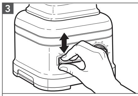
Flip the START/STOP toggle switch up or down to begin operation of the Blender. The Status Indicator Light will now be solid.
