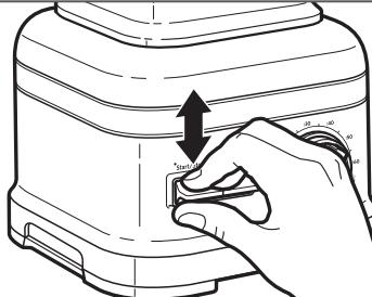
After blending, flip the START/STOP toggle switch up or down. Allow the Blender to come to a complete stop before removing the Lid and pouring your blended ingredients.
