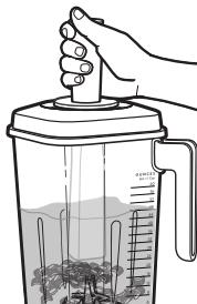
Utilize the Flex Edge tamper accessory as needed for optimal blending performance. Remove the Ingredient-measuring Cap only, and leave the Lid in place. Stir or press contents down towards the blade. When you are finished, replace the ingredient-measuring cap in the Blender Jar Lid before resuming blending.
