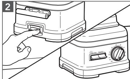
The main power switch is on the back of the Blender Base. Flip the POWER switch to the ON (I) position. The Status Indicator Light above the Start toggle button will begin to flash, indicating that the Blender is in Standby mode. The Blender is now ready to operate.
