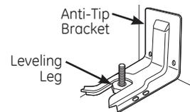
To reduce the risk of tipping the range, the range must be secured by a properly installed anti-tip bracket. See installation instructions shipped with the bracket for complete details before attempting to install.
