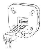
Figure 5 Installing the removable connector
