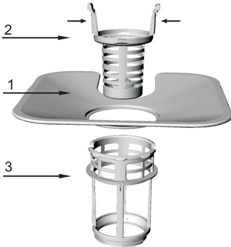
The filter system consists of a coarse filter, a flat (Main filter) and a micro filter (fine filter).
