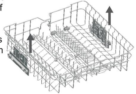
In loaded basket adjustment mechanism, make sure that both sides are in the same position (up or down).
