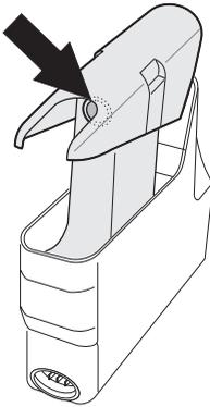
If the connection valve becomes brittle, dried out or if a lot of water collects at the bottom of the steam connector niche, the valve needs to be replaced.
