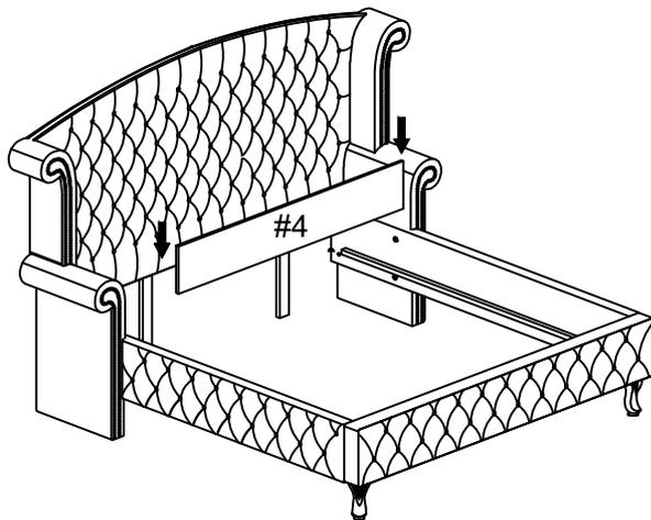
Align HB panel (#4) to the headboard, then secure by using screws (#J).
