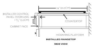
10" (25.4CM) TO COMBUSTIBLE SIDE WALL MIN. BOTH SIDES 11/2" (3.8CM) TYPICAL COUNTERTOP THICKNESS 1/<sub>2</sub>" (1.3CM) OVERHANG, **BOTH SIDES** 0 0 (19.7CM) 0 0 36" (91.4CM) TYPICAL (2.5CM) MIN THICKNESS CABINET / COUNTERTOP DIMENSIONS
