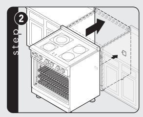
Slide range into place. Be sure anti-tip bracket slides into the anit-tip opening.
