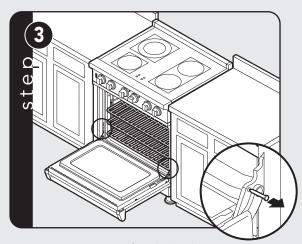
Remove pins from hole in hinges.
