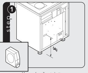
Measure from floor to bottom of the anit-tip opening located on the back of range.
