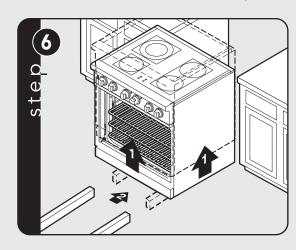
Lift unit and prop on wood blocks.
