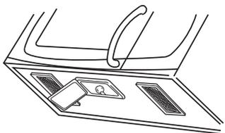
3. Replace the bulb with a 30 watt appliance bulb.
