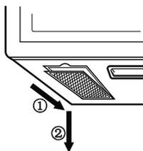
2. Soak grease filters in hot water and a mild detergent. Rinse well and shake to dry. **Do not use ammonia or place them in a dishwasher. The aluminum will darken.**
