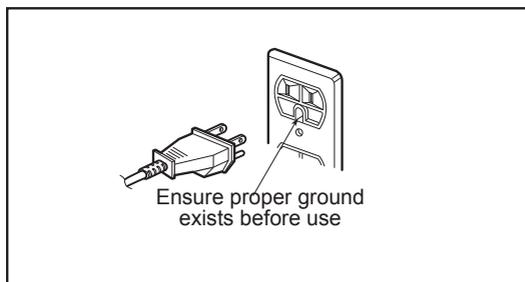
For a permanently connected appliance: This appliance must be connected to a grounded, metallic, permanent wiring system, or an equipment grounding conductor should be run with the circuit conductors and connected to the equipment grounding terminal or lead on the appliance.
