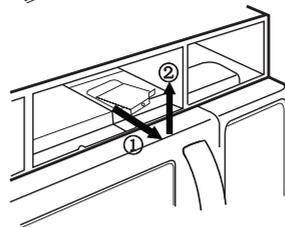
5. Replace the bulb with a 30 watt appliance bulb.
