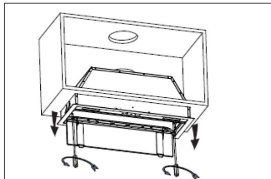
4. Use the screwdriver to take out the screws that connects the panel to the cabinet.
