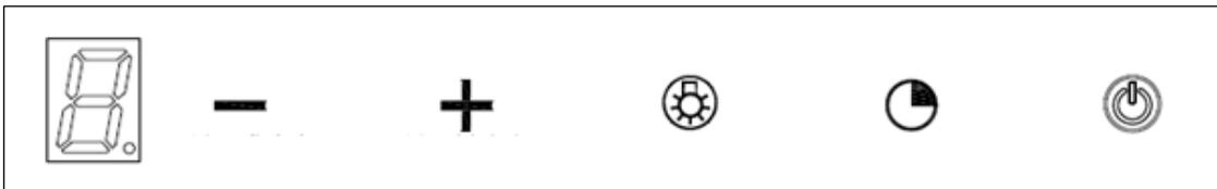
**POWER** : once the hood is connected to the main supply, the backlight will be turned on, output will be closed and the unit will enter into a “stand-by” mode.
