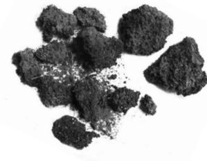
*Above is an example of a pellet “clinker”. This mass of impurities can reduce airflow through the burn pot and create an unsafe burning condition.*
