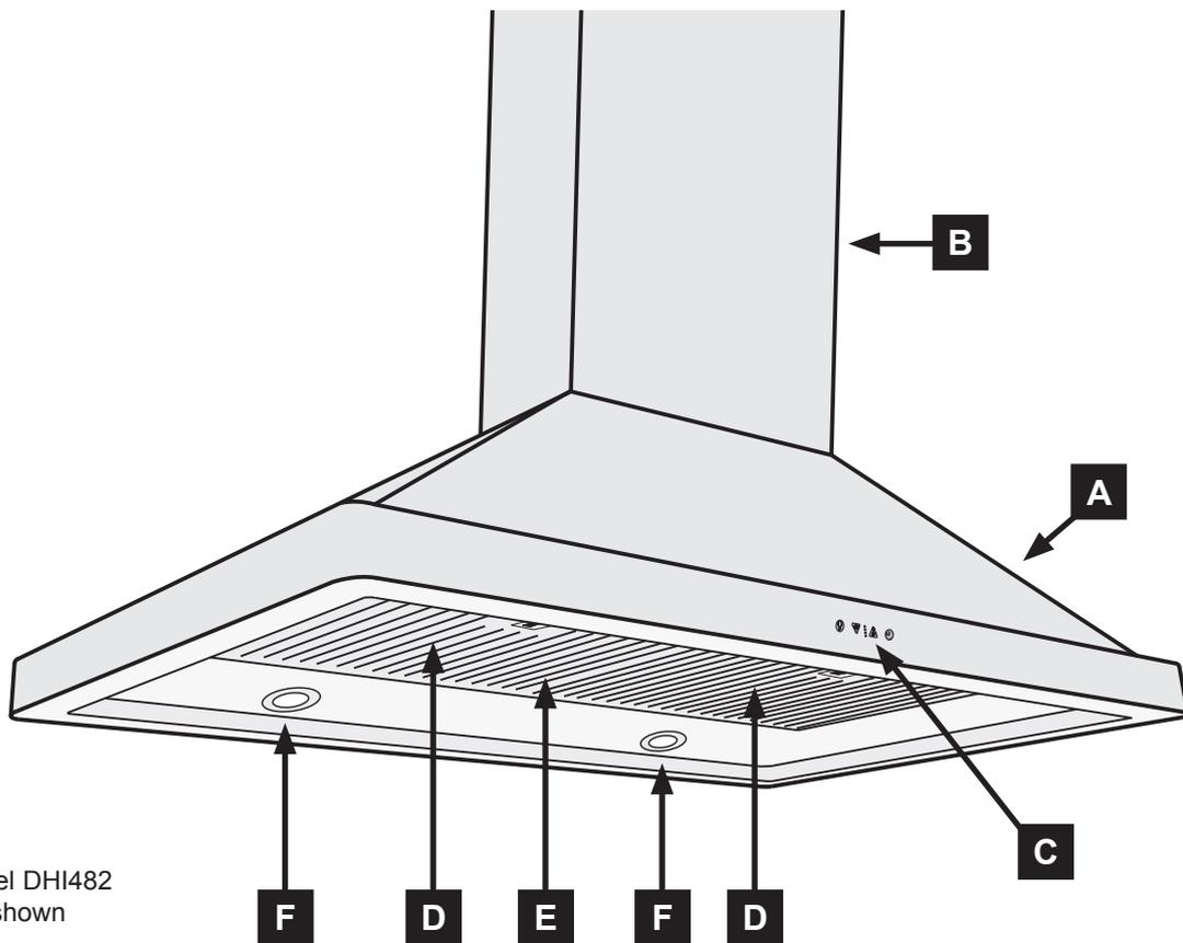
**A HOOD** - The hood directs heat and smoke into the blower system located inside the unit. The blower system forces heat and smoke into the duct inside the chimney **B** which vents to the outside. The filter(s), the lights and main power switch are located on the under side of the hood. The blower system on some hoods consists of two blowers. See the table below.
