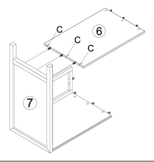
Step 6 Insert screw B (x1), C (x3) Cam lock D (x3) into parts (6),(8).
