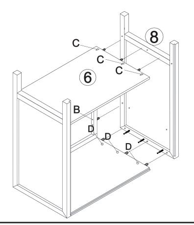
Step 7 Insert screw B (x4) into parts (5).
