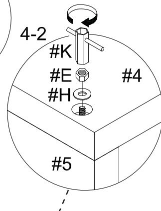
2. Carefully place the bottom shelf (#4) onto each rod and wood dowels. Apply a flat washer (#H) then a hex nut (#E) onto the ends of the rods. Secure using the socket wrench (#K).
