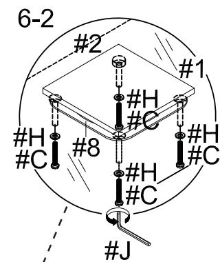
2. Prepare 4 bolts by inserting a flat washer (#H) onto the bolts (#C), then from below insert into the holes along the top panel (#2). Secure using the Allen wrench (#J).
