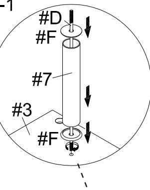
1. Insert the threaded end of a rod (#D) into the single hole, turn right to tighten. Then insert a cap (#F), support tube (#7), and another cap (#F) in that order onto the rod (#D).
