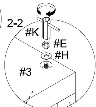
2. Carefully place the middle shelf (#3) onto each rod and wood dowels. Apply a flat washer (#H) then a hex nut (#E) onto the ends of the rods. Secure using the socket wrench (#K).
