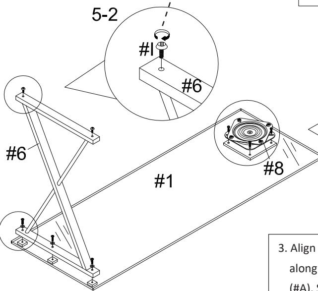
3. Align the spin hinge (#8) to the holes along the glass top, then insert 4 bolts (#A). Secure using the Allen wrench (#J).
