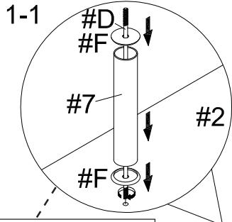
1. Insert the threaded end of a rod (#D) into the single hole, along the top panel (#2) turn right to tighten. Then insert a cap (#F), support tube (#7), and another cap (#F) in that order onto the rod (#D).
