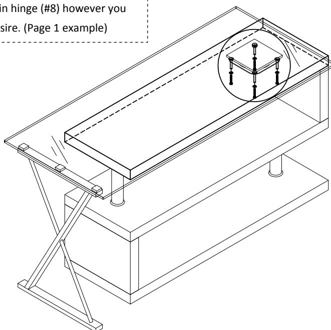
1. Turn the glass top upright, then align the spin hinge (#8) to the holes along the top of the top panel (#2)
