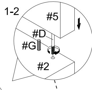
2. Insert the rods (#D) into the outer holes, turn right to tighten. Insert the wood dowels (#G) into the inner holes. Then apply the side panel (#5) onto the rods and wood dowels.
