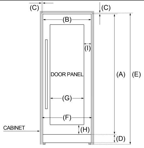
NOTE: The wine column comes with a 4" (100 mm) stainless steel toe kick installed to fit a standard 84" (2134 mm) tall cabinet niche. For flush installation in a standard 25" (635 mm) deep cabinet niche, maximum door panel thickness is 3/4" (19 mm).
