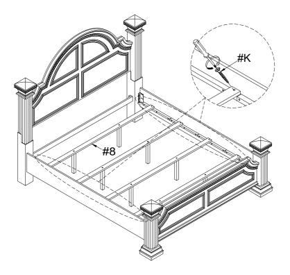
Align slats (#8) to the side rails, then secure by using screws (#K).
