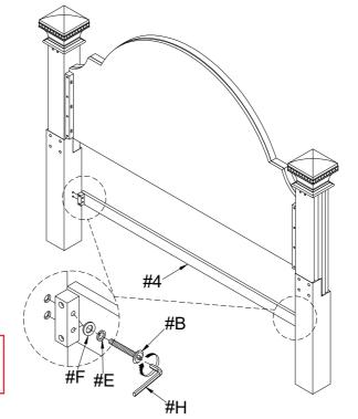
Align HB support (#4) to the HB legs, then secure by using bolts (#B) with washers (#E,F).
