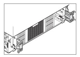
Insert the base cover retainers on both sides into the appliance housing.
