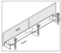
Securing to a concrete floor using the supplied concrete anchors.
