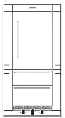
Use only the matching base cover with the ventilation slits! If there is insufficient ventilation, the compressor will run more often and over a longer period of time. This results in higher energy consumption and a higher compressor temperature which can damage the compressor.
