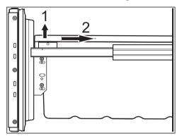
■ Lift the container at the front left and right (1) and push it slightly backwards (2).
