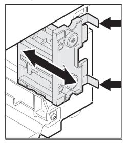
■ The face end of the angles on the retainers must be flush with the front of the toe-kick cover. If this is not the case, adjust the retainers according to the depth.
