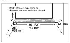
The anti-tip bracket must be level after installation even if the floor is not level. Install the wooden spacer in an appropriate position.
