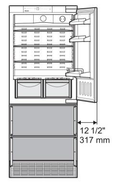
These measurements do not take the cabinet front and the door handle into account; they must be added on accordingly.
