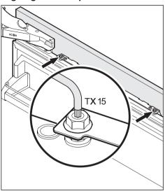
To vertically align the door panel with the adjacent cabinet doors,
