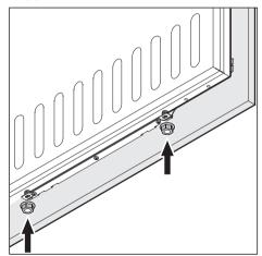
■ Screw the nuts onto the adjustment bolts and tighten them.
