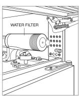
Water filter cartridge removal.
