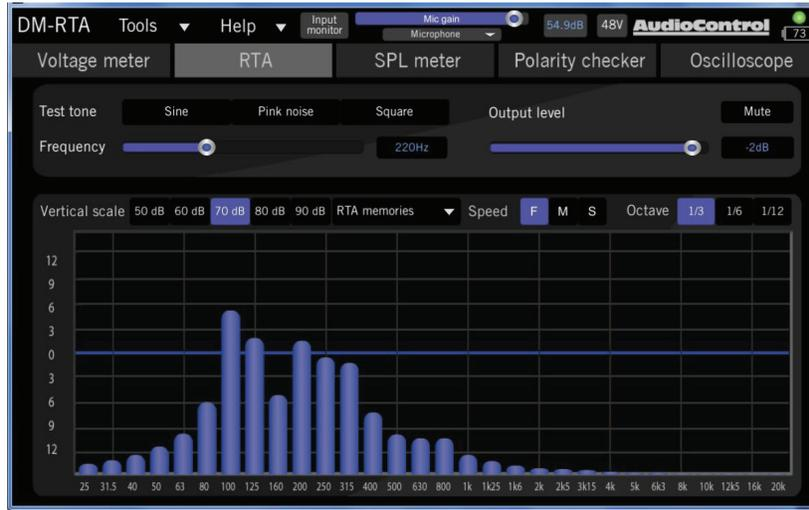
The RTA display allows you to see the response of your system, and see how the levels vary across the audio range of frequencies. You can investigate any gaps in the response, adjust crossover controls (if your system allows such niceties) and adjust any EQ controls you might have.
