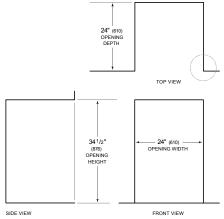
NOTE: 3<sup>1</sup>/2" (89) finished returns will be visible and should be finished to match cabin
