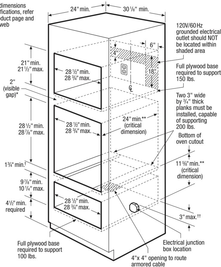
\* Minimum 2 1/8" clearance required from bottom of Built-In Microwave cutout to top edge of Wall Oven's faceplate, leaving a 2" visible gap between both product faceplates.
