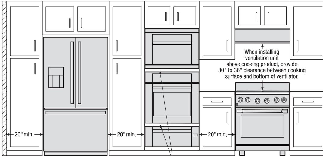
When installing appliances adjacent to each other, 20" minimum distance between each appliance required.
