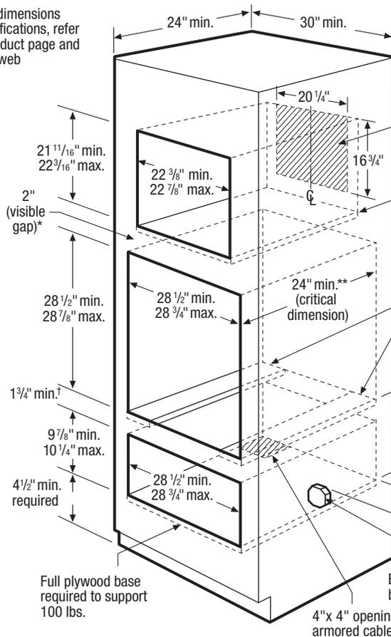
240V/60Hz grounded electrical outlet should NOT be located within shaded area
