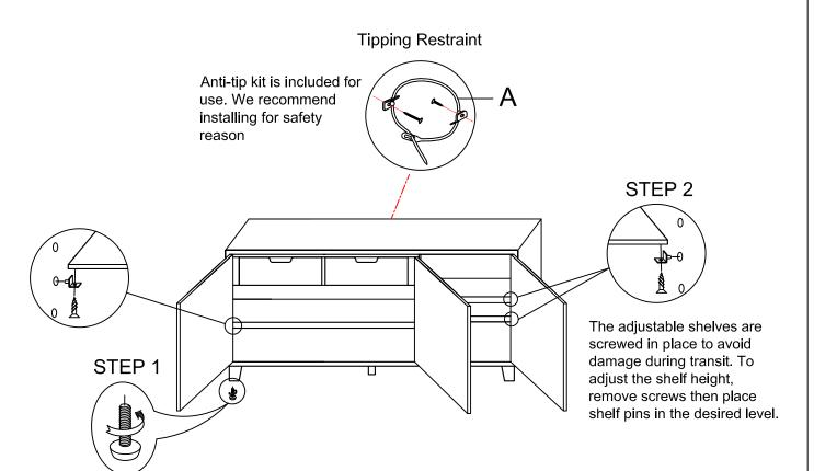
Adjust Leveler if needed to level buffet on uneven floor.
