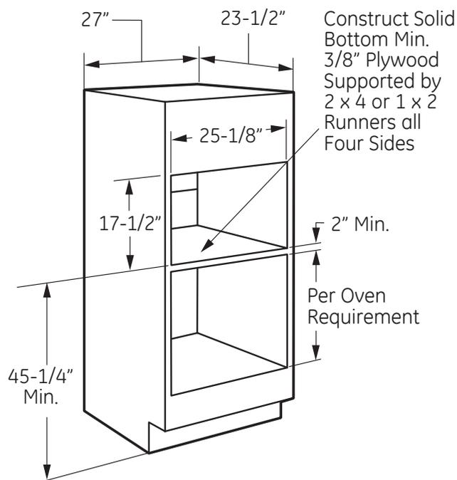
\*If you are replacing a GE electric double oven with the combined installation of an Advantium 120 and a single oven, use the dimensions shown. The middle rail separating the two openings may need to be larger than the 2" minimum shown.
