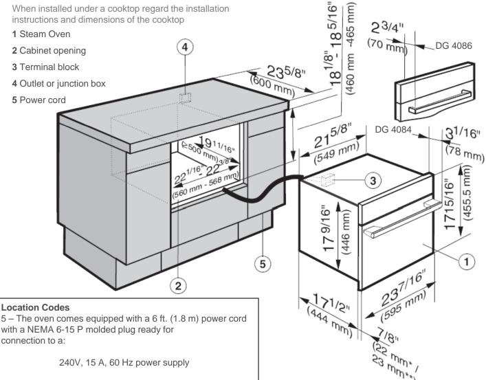
4 – 2 ½ <sup>2</sup> minimum hole size for plug. Outlet to be installed in adjacent cabinetry
