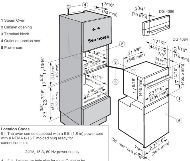
$4-2\frac{1}{2}$  minimum hole size for plug. Outlet to be installed in adjacent cabinetry
