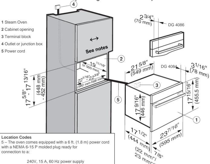
$4-2\frac{1}{2}$  minimum hole size for plug. Outlet to be installed in adjacent cabinetry
