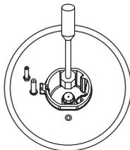
4. Replace the injectors with those supplied corresponding to the gas available (see Burner and Injector Characteristics table).
