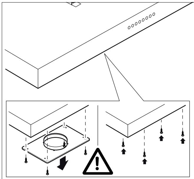
Slide the remote fan unit into the ventilation hood from above. Use four screws to secure it in place.
