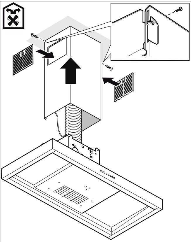
**3 Fit the lower flue duct.**
