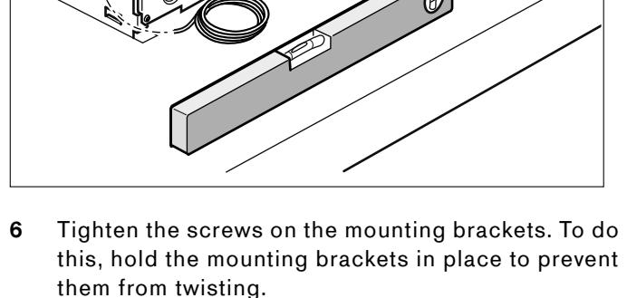
6 Tighten the screws on the mounting brackets. To do this, hold the mounting brackets in place to prevent them from twisting.
