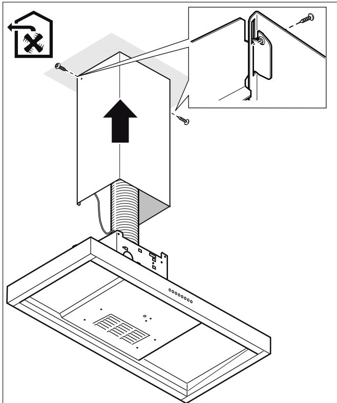
**4 Place the lower flue duct on the appliance.**
