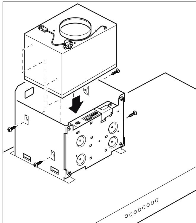
Connect the mains cable and control cable to the control module.
