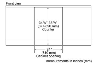
Thermador double drawer under counter top dimension. (Unit door flushed with the cutout) measurements in inches (mm)
