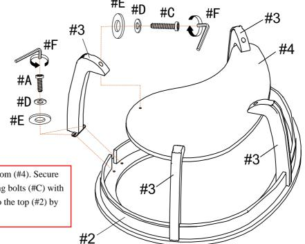
Align feet (#3) to the top (#2) and bottom (#4). Secure the feet (#3) to the bottom (#4) by using bolts (#C) with washers (#D,E). Secure the feet (#3) to the top (#2) by using bolts (#A) with washers (#D,E).
